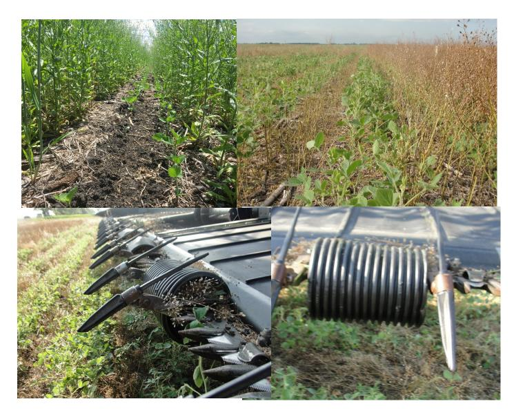
Fig. 36. Top left, interseeded soybean into standing winter camelina; Top right, winter camelina harvest (left harvested); Bottom left, combine header adapted to avoid cutting soybean plants while harvesting camelina; Bottom right, drainage tile pipe over cutter bar to protect soybean plants during camelina harvest.
