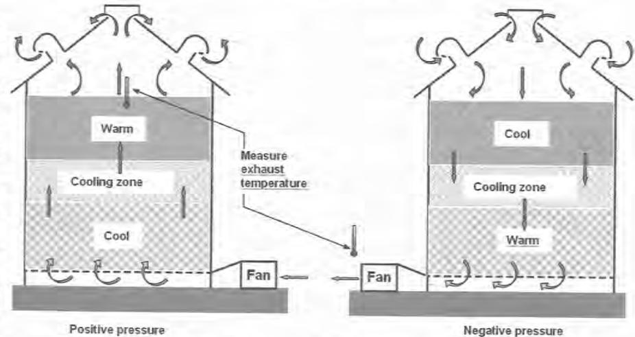
Figure 2.5 Movement of cooling zones during grain aeration.
