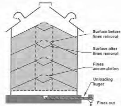
Figure 2.1 Removal of accumulated fines during bin filling.
