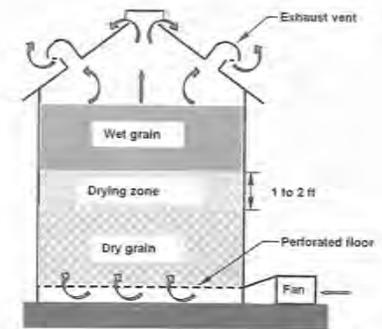
Figure 2.2 Illustration of a natural-air drying bin.
