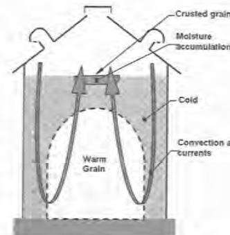
Figure 2.3 Moisture migration in grain that has not been adequately cooled.
