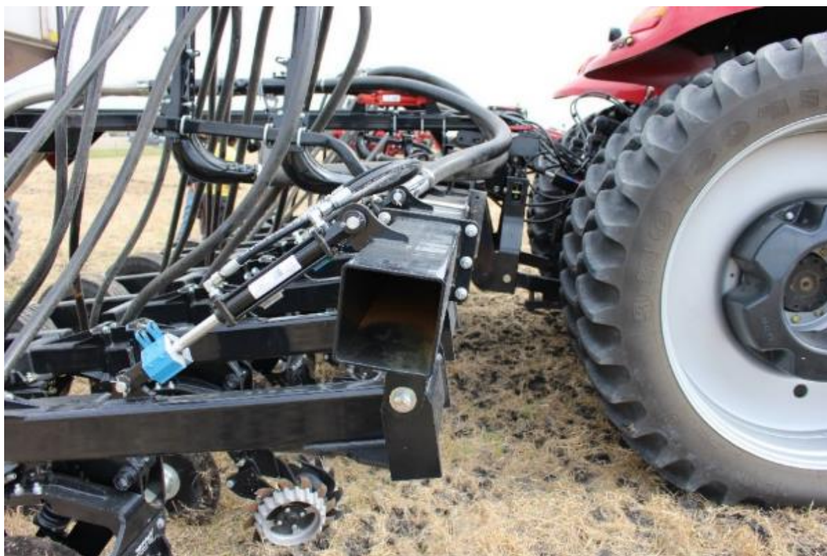
Fig. 1. Pilot twin row planter developed by Amity Technology International for the project. Photo Karen Hertsgaard
