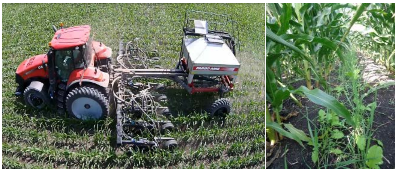
Fig. 2. New interseeder planting cover crops at V6 stage (Photo: Abbey Wick). Rye and radish established with the interseeder. Photo taken August 16 (Photo: M. Berti)
