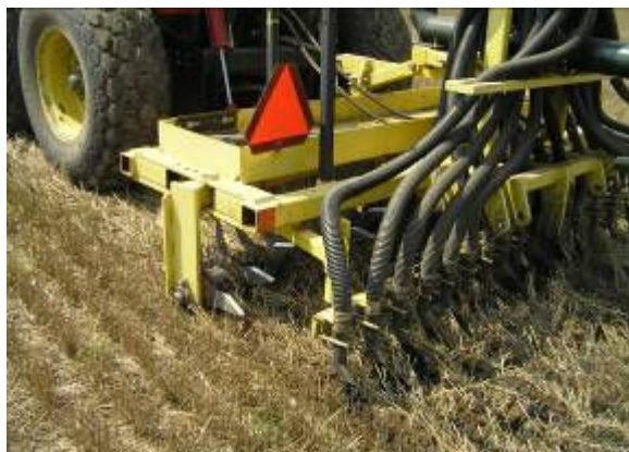
Figure 1. The rolling-tine aerator created cracks and fissures in the untilled ground and the drop tube applicator placed the seed-laden slurry in the fractured soil.
